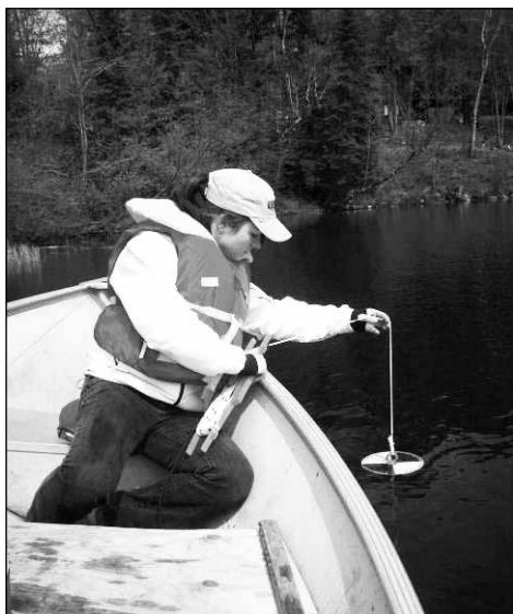
A volunteer uses a Secchi disc to record water transparency.
