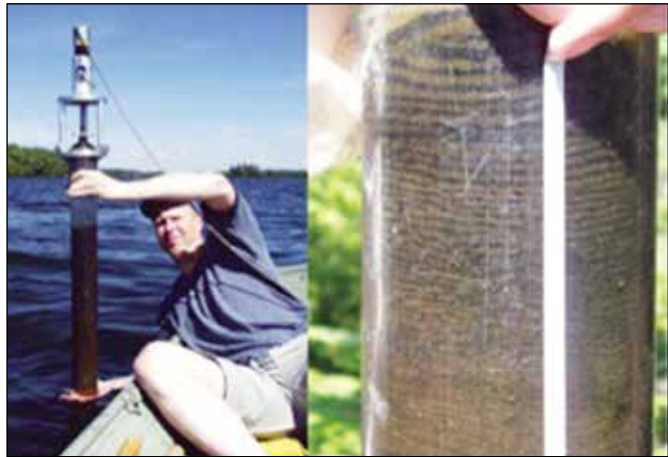
Fig. 3. A simple Grew gravity corer is shown on the left. The amount of weight used on a gravity corer largely depends on the water content of the sediments and the nature of the organic and inorganic matter. The close-up of a core on the right (taken from northwest Ontario, Arpin Lake), shows the sediment structure that can be recovered with this simple coring device. In this case the alternating light and dark layers represent an annual deposition of sediment (termed a varve).
