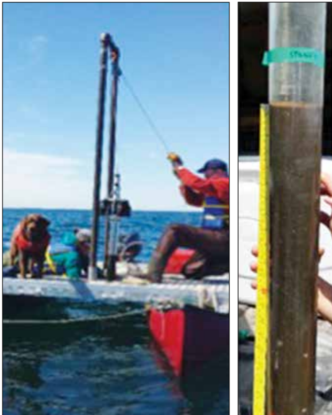
Fig. 3. Coring platform used in this project. The platform is mounted across two structurally-reinforced canoes. The Glew gravity corer was equipped with an 80-cm core tube, and weighs approximately 28 kg. The chocolate Lab Sasha is wearing a Ruffwear life jacket. The sediment core from Stony Lake is shown on the right.
