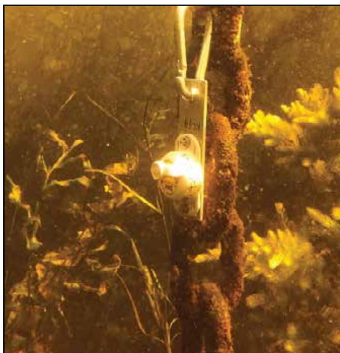
Figure 2. A water temperature logging device deployed in mid-lake in summer 2022, to track hourly temperatures on an annual basis.
